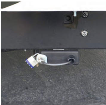
Toy Lock with a 15 foot steel braided cable that is secured to the frame. This allows you to lock up your toys at night or when away from camp, knowing your belongings are secure.
