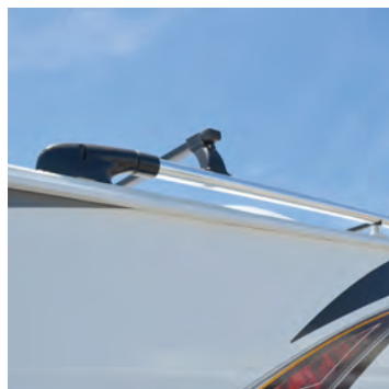
Roof Rack System is frame mounted to carry more gear and compatible with many aftermarket components such as storage pods, paddle/surf board/kayak racks and others.
